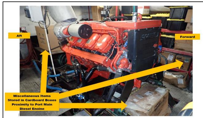
Figure 4: Combustible materials stored in the engine room.
